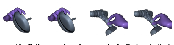
Figure 10: Failure modes of our method. Each pair displays a sample from dual views. The left side shows a generated grasp appears to be more of a touch rather than a proper grasp. The right side shows an unsatisfactory grasp when the sampled ContactGen is infeasible on out-of-domain objects.
